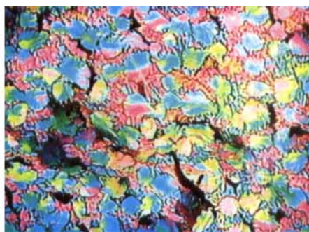
Figure 7. (a) Optical micrograph of the PEO/PAA 20/80 blend at 384 K, showing the formation of nematic droplets of PAA on cooling from the isotropic phase (crossed Nicols, \times 100 ). (b) Optical micrograph of the PEO/PAA 20/80 blend after cooling to 303 K (crossed Nicols, \times 100 ).
